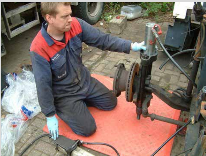
Assemble the KPP20, push the hydraulic pump – the pin pops out. Job done!
