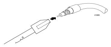
Push the flare/calibration tool gently and rotate slightly onto the connector while applying pressure. This will work the base of the connector underneath the wire braid slowly.
