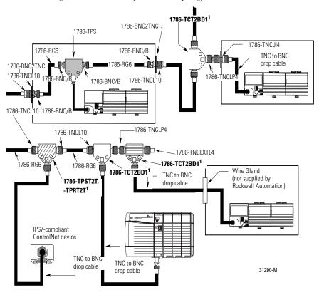
1 Although the arrow in this illustration points to the tap body, the catalog number called out corresponds to the appropriate ControlNet Tap and Cable Assembly Kit.
